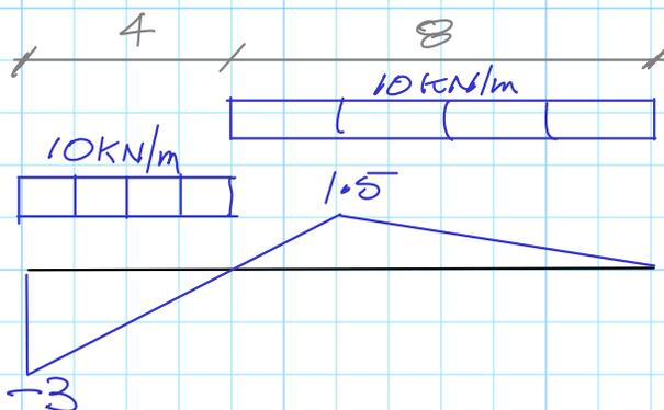
$$M_c^- = 10 \times -3 \times 4 \times \frac{1}{2} = -60 \text{ kN-m}$$
