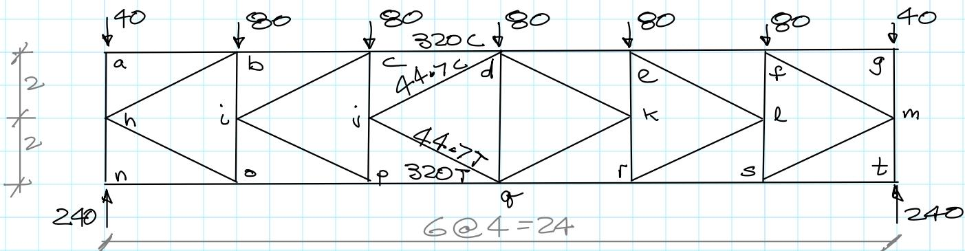
Note: diagonals resist shear force, which is small near centre span.
