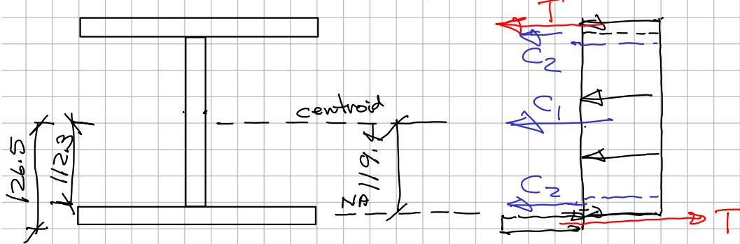
$$\begin{aligned}C_1 &= \text{compression in web} \\&= 224.6 \times 8.6 \times 345 \times 10^{-3} \\&= 666.388 \text{ kN}\end{aligned}$$
