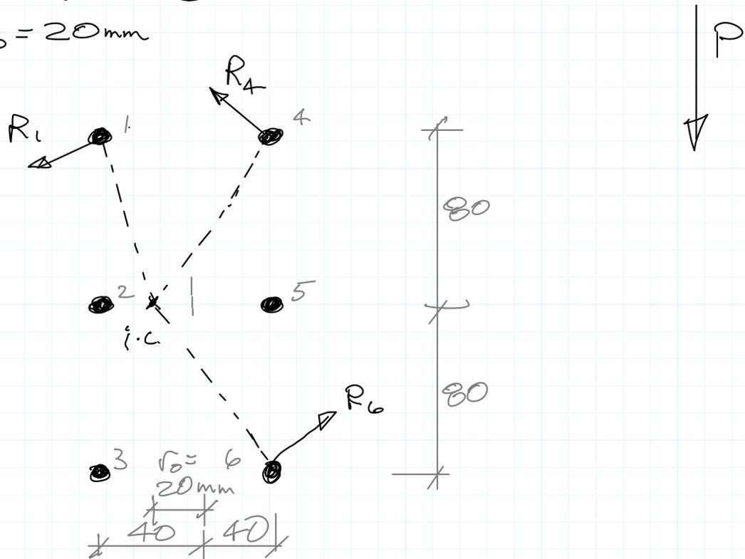
Assume that one plate rotates rigidly about i.c. Then shear deformation in each bolt is proportional to distance from i.c.
